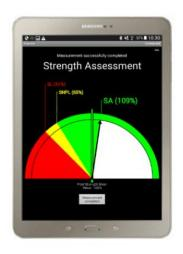
The new improved CXI-PT5500 graphical interface is now properly working with Telecom and Electricity wooden poles. The changes to the new GUI allow the operator to configure Utilities Poles with several functions, like Extra High Voltage Poles, High Voltage Poles, Low Voltage Poles, Telecom Poles, and poles with mixed configuration, for example equipped with CaTV and Fiber Optic cables.
