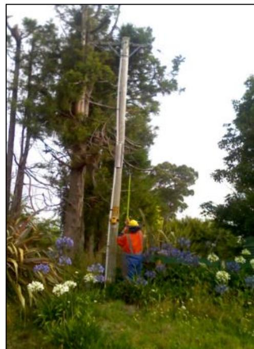
Finally, the CXI-PT5500 test result (Strength Assessment SA) and the lab UBS have been compared, for all poles of the considered set. As a result of this comparison, it has been verified that the SA is always equal to or smaller than the actual strength measured in the lab, so being the CXI-PT5500 result always in favour of safety, and this is consistent with the goal of the algorithm to always take decisions on the safety side.
