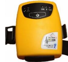
Cinetix/Vonaq tool has been successfully tested by PowerCo, a New Zealand Power Company that decided to run a Field Trial to test the capability of Cinetix/Vonaq CXI-PT5500 Pole Tester to estimate wooden poles Ultimate Breaking Strength (UBS), namely the pole maximum bending load before breaking.
